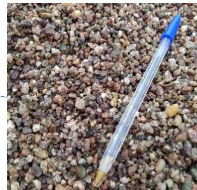
Massif filtrant (gravillons)
