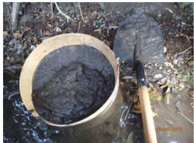
Figure 24 : Excavation du substrat - S=0.5m 2
